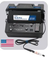
emission heated diode with audible and visual leak rate indicators. It is the most sensitive and accurate leak detector to detect all CFC, HFC and HCFC refrigerants as low as 0.006 oz/yr, including R-410a and R-507. The unit is mounted in a durable carry case which houses the 4.5 foot probe with built in filter, carrying strap, wall adapter and operating instructions.
